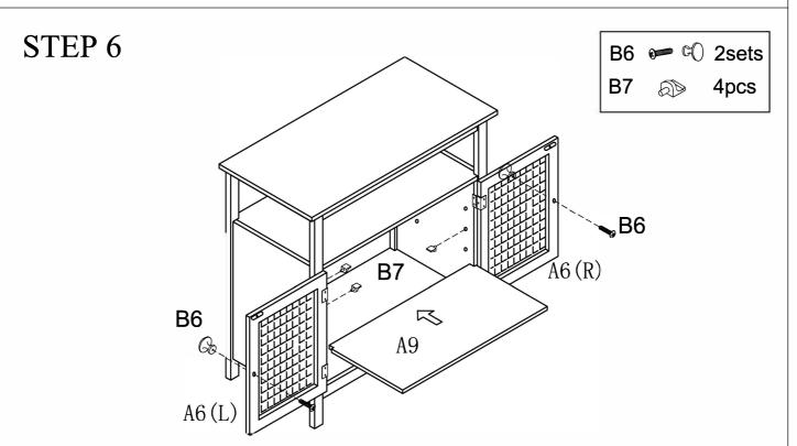
Insert Shelf Supports B7 into the holes of Side Panels A2, then place shelf A9 onto Shelf Supports B7.
