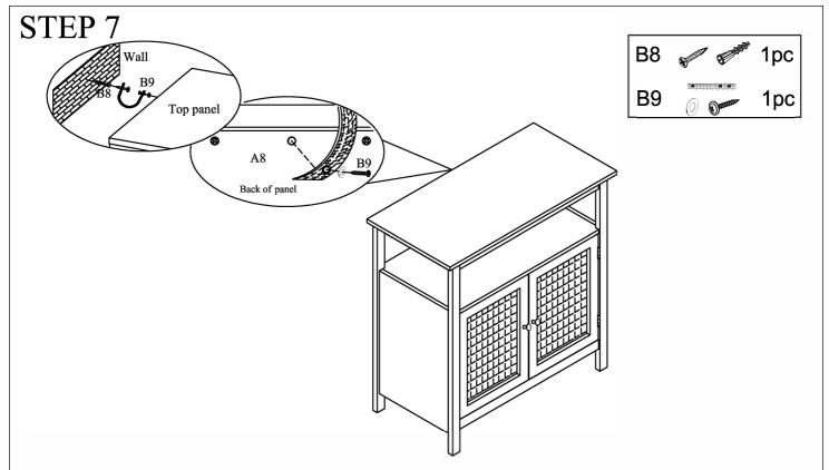
For your safety, please attach unit to the wall by Anchor with screw B8 and Antitip kit B9.
