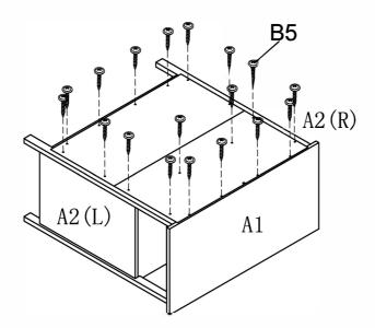
Attach Back Panel A8 to the back of unit using Screws B5.
