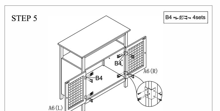
Assemble Doors A6 to Side Panels A2 using Hinge with Screws B4.
