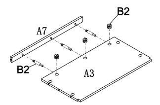
Assemble Apron A7 to Bottom Panel A3 using Camlocks B2.
