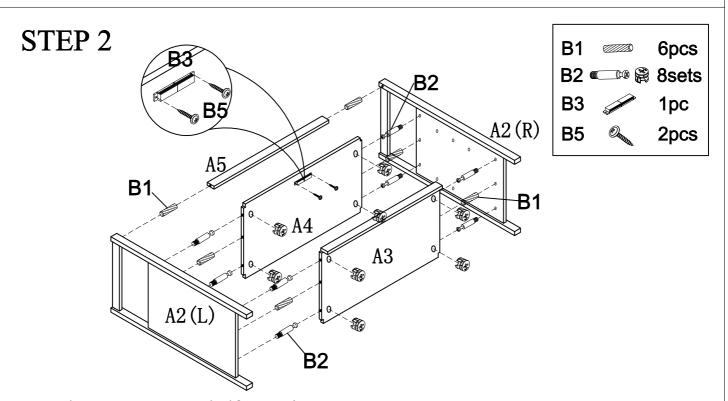
Attach Magnet B3 to Shelf A4 using Screw B5.
