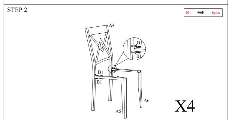
Assemble Legs A5&A6 to Back Frame A4 using Bolts B1. Noted:Please do not tighten Bolts B1 until Step 4.
