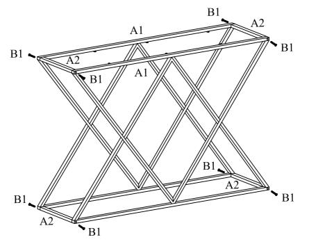
Assemble Frames A1 to Connect Bars A2 using Bolts B1. Noted:Please do not tighten Bolts B1 until Step 2.
