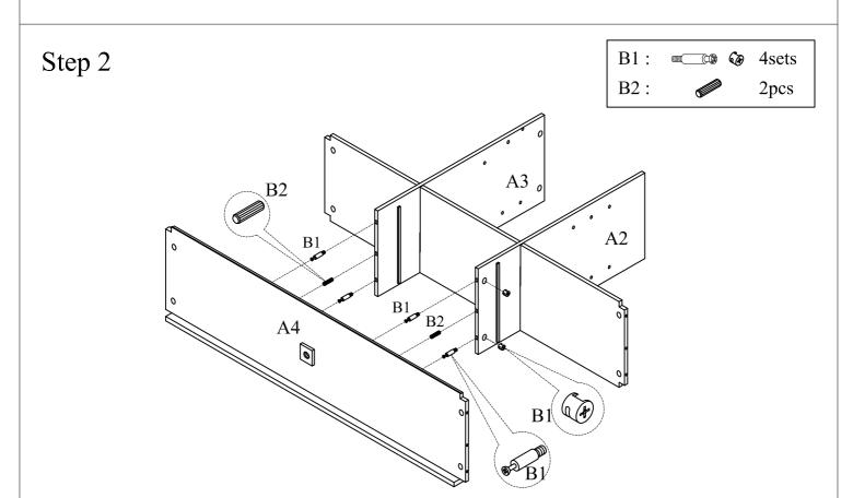
Assemble Bottom Panel A4 to Middle Dividers A2 & A3 using Camlocks B1 and Wood Dowels B2.
