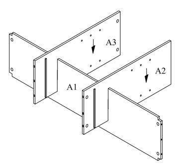
Insert Middle Dividers A2 & A3 into the grooves of Middle Shelf Panel A1 as shown above.
