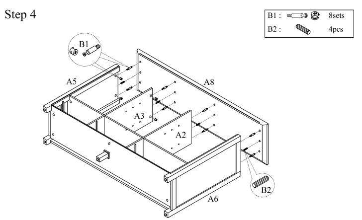
Assemble Top Panel A8 to Middle Dividers A2 & A3 and Side Panels A5 & A6 using Camlocks B1 and Wood Dowels B2.
