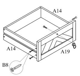
Assemble Right Drawer Front Panel A18 and Center Drawer Front Panel A19 to Drawer Side Panels A14 using Screws B8,then attach Handles B9 to Drawer Front Panels A18 & A19 using included bolts.
