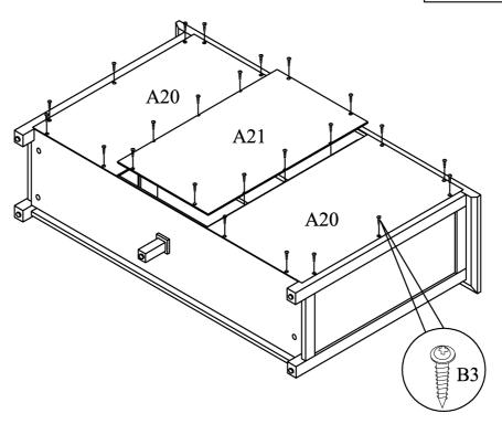
Assemble Back Panels A20 and Center Back Panel A21 to the back of this unit using Screws B3 as shown above.
