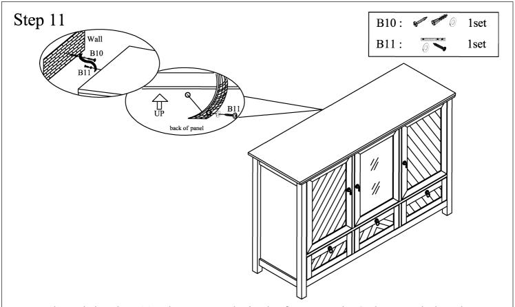
Attach Anti-tip Kit B 11 nylon strap to the back of Top Panel A8, then attach the other end of the nylon strap to the wall using Anchor and Screw B 10 as shown above.
