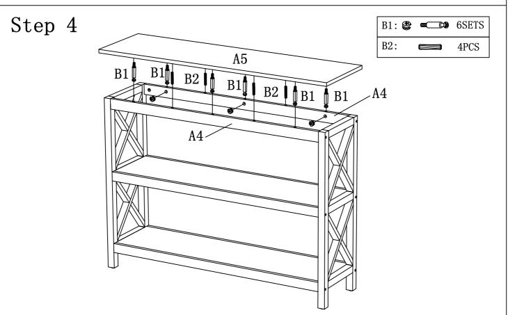
Attach Top Panel A5 to Connect Bars A4 using Cambolts&Camlocks B1 and Wood Dowels B2.
