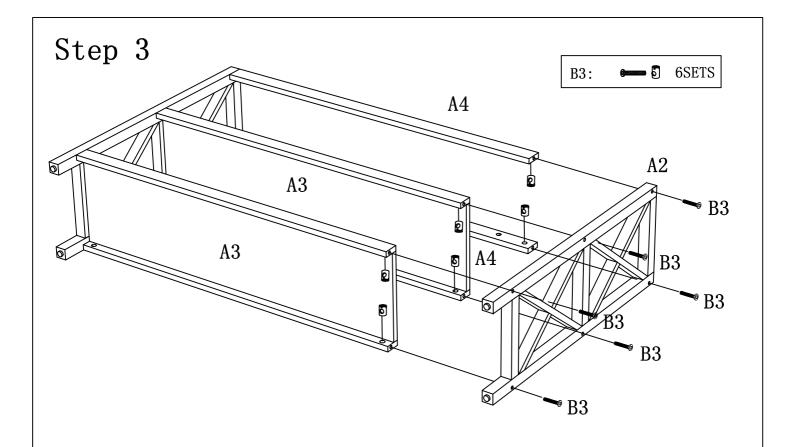
Attach Right Frame A2 to Connect Bars A4 and Shelf Panels A3 using Bolts B3 with Nuts.
