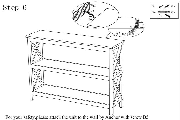
For your safety, please attach the unit to the wall by Anchor with screw B3 and Anti-tip kit B6.
