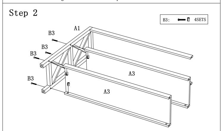
Attach Shelf Panels A3 to Left Frame A1 using Bolts B3 with Nuts. Note: Please do not tighten Bolts B3 until Step 4.
