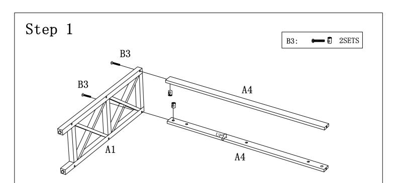
Attach Left Frame A1 to Connect Bars A4 using Bolts B3 with Nuts. Note: Please do not tighten Bolts B3 until Step 4.
