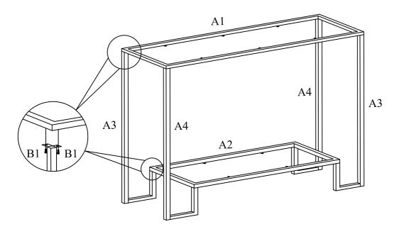
Assemble Frames A1&A2 to Legs A3&A4 using Bolts B1 as shown above. Noted:Please do not tighten Bolts B1 until Step 2.
