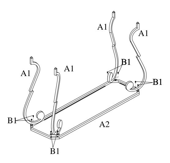
Assemble Legs A1 to the Top Frame A2 using Bolts B1. Note: Please do not tighten bolts B1 until Step 3.
