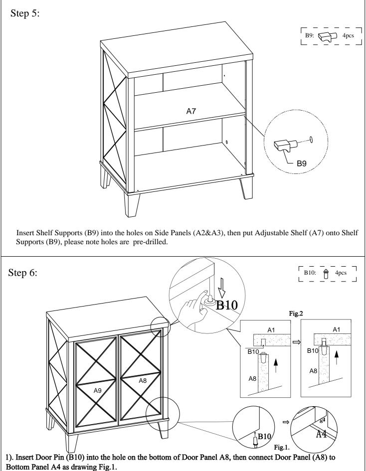
2). Insert Door Pin B10 into the hole on the top of Door Panel (A8), then press down Door Pin B10 ( see Fig.2.) and hold the door panel carefully into the cabinet with the door pin poping up into the hole of Top Panel (A1).
