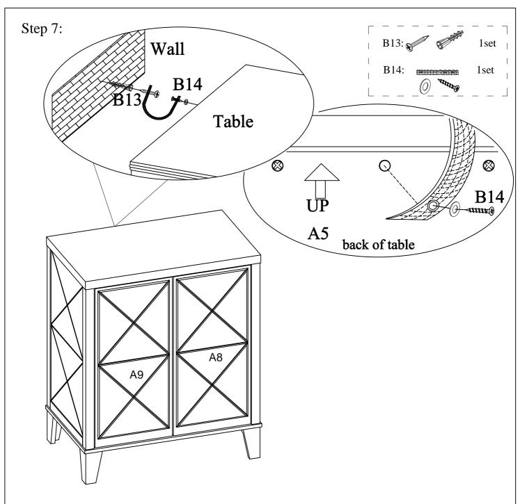
For your safey, please attach this unit to the wall by Anti-tip Kit B14 and Anchor with screw B13.
