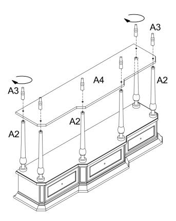
Attach Bottom Legs A3 by inserting legs through the Bottom Panel A4 and attaching it to Middle Legs A2.
