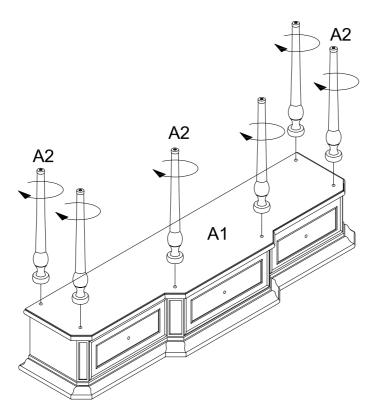
Attach and tighten Middle Legs A2 to Top Part A1 as shown above.
