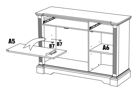
Insert Shelf Supports B7 into holes on Side Panels A1 & A2, Divider A9, then put Shelves A5 & A6 onto Shelf Supports B7 as shown above.
