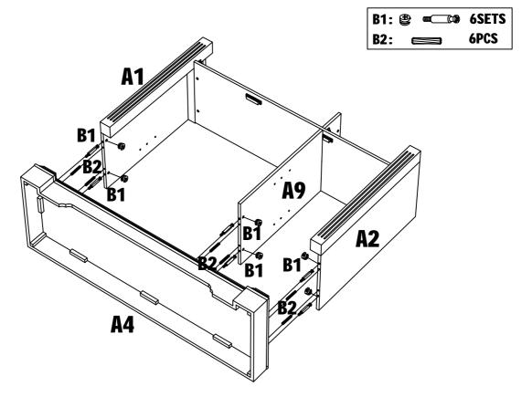
Assemble Side Panels A1 & A2 to Bottom Panel A4 using Camlocks B1 and Wood Dowel B2 as shown above.
