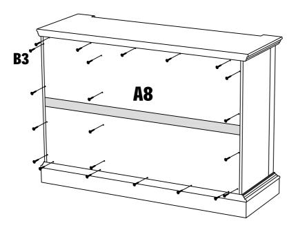
Attach Back Panel A8 to the back of the unit using Screws B3 as shown above.
