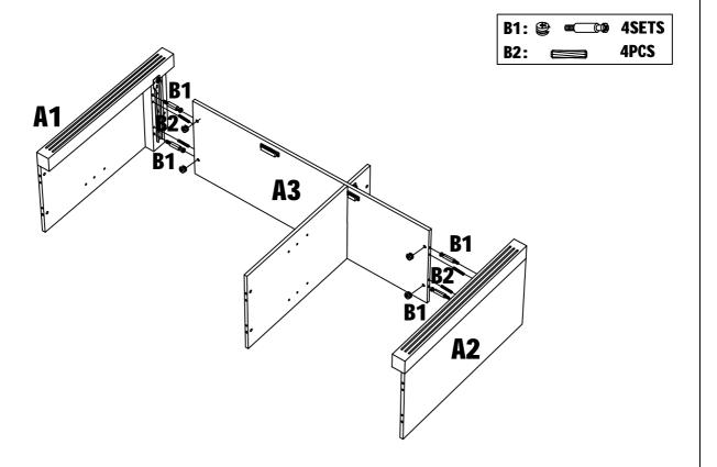
Assemble Side Panels A1 &A2 to Divider A3 using Camlocks B1 & Wood Dowels B2 as shown above.
