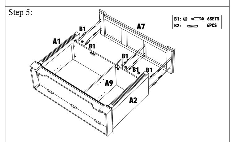
Assemble Side Panels A1 & A2 to Top Panel A7 using Camlocks B1 and Wood Dowel B2 as shown above.
