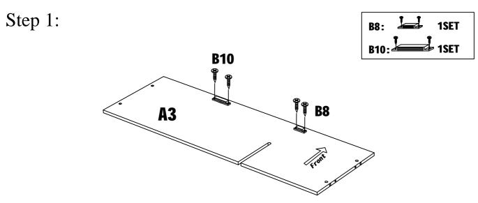
Assemble Magnets B8 & B10 to Divider A3 using included screws. Note: Holes are pre-drilled.
