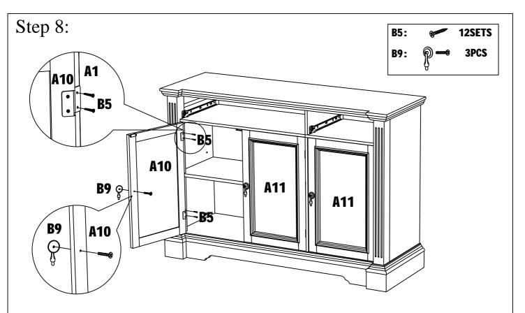
Assemble Left Door A10 to Side Panel A1 using Screws B5 as shown above. Then attach Handle B9 to Left Door A10 using included bolt.
