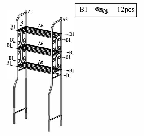
Attach Racks A6 to Side Frames A1&A2 using Bolts B1. Please do not tighten Bolts B1 until step 5.
