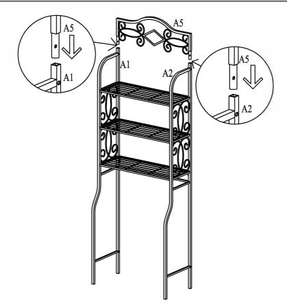
Insert Back Frame A5 into Side Frames A1&A2 as shown above.
