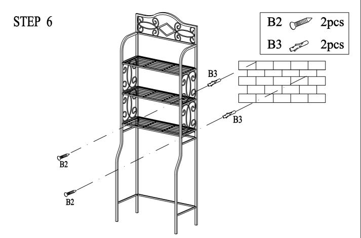
For your safety, please attach this unit to the wall with provided Anchors B3 and Screws B2.
