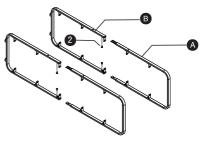
Attach Connnecting Bars (C) to the back of Lower Frames (A) Attach Shelf Panels (D) to Lower Frames (B) and Upper (B) and Upper Frames (A) using Bolts(1) as shown below. Note:Do not tighten Bolts(1) until Step 4.
