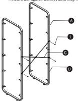
Frames (A) using Bolts(1) as shown below. Note:Do not tighten Bolts(1) until all panels are attached.
