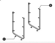
2 Tighten and Insert Upper Frames(A) into Lower Frames (B) using Bolts(2).
