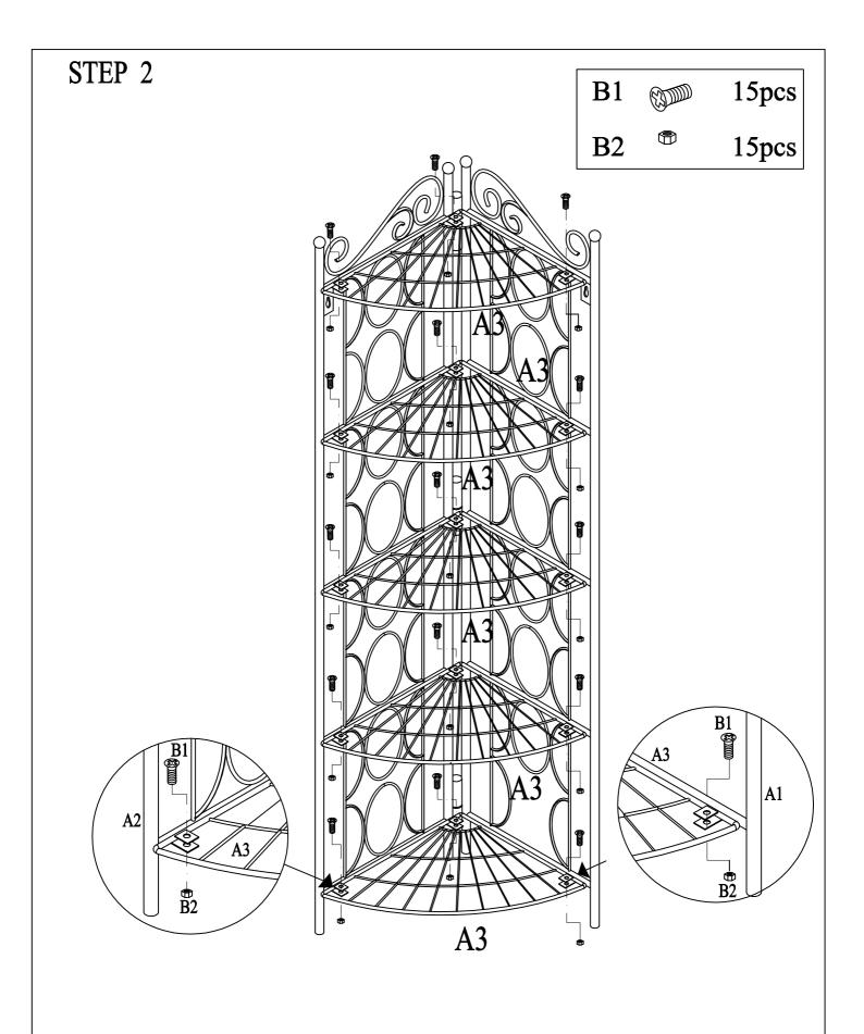
Assemble Net Racks A3 to Side Frames A1&A2 using Bolts B1 and Nuts B2.
