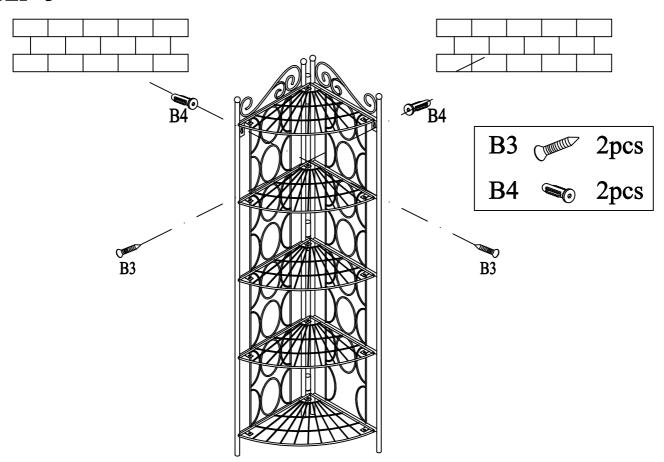
For your safety, please attach this rack to the wall by using Screws B3 and Anchor B4 as shown above.
