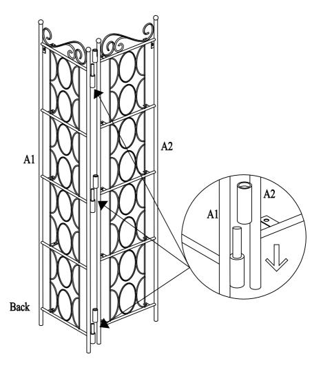
Insert Left Side Frame A2 onto Right Side Frame A1 as shown above.
