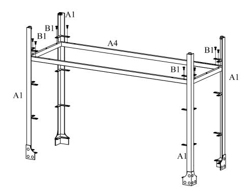
Assemble Legs A1 to Shelf Frame A4 using Bolts B1, do not tighten Bolts B1 until Step 9.
