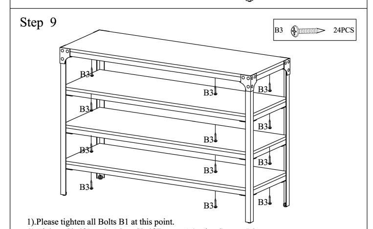
2). Tighten Shelf Panels A5 to Shelf Frames A4 using Screws B3.
