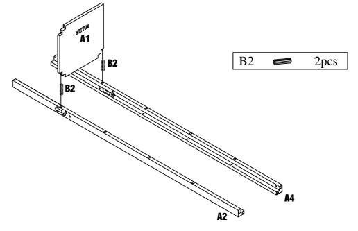
Assemble Legs A2 & A4 to Shelf A1 using Wood Dowels B2.
