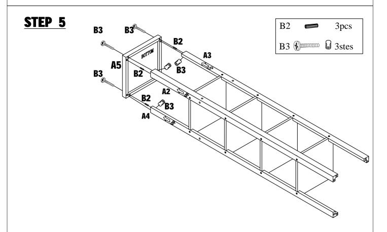
Assemble Legs A2 & A3 & A4 to Top Panel A5 using Bolts with nut B3 & Wood Dowels B2 as shown above.
