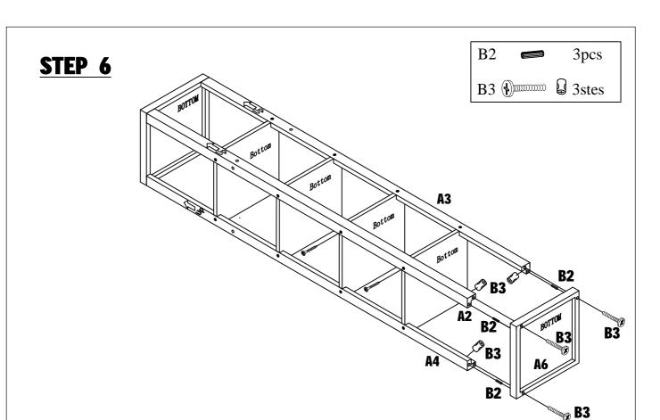
Assemble Legs A2 & A3 & A4 to Bottom Panel A6 using Bolts with nut B3 and Wood Dowels B2 as shown above.
