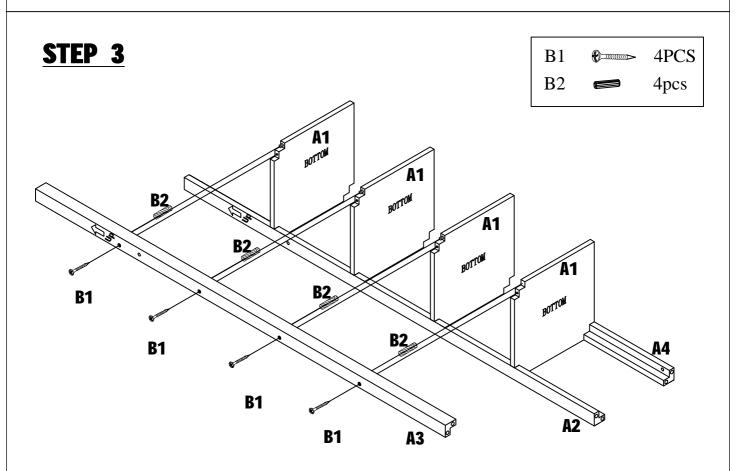
Assemble Left Leg A3 to Shelves A1 using Wood Dowels B2 and Screws B1 as shown above. Note: Please make sure Shelves A1 exactly inserted into the grooves on Left Leg A3.
