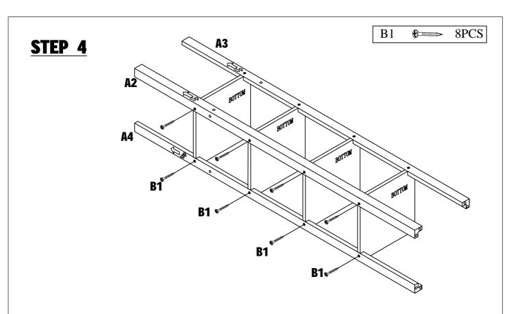
Tighten Legs A2 &A4 to Shelves A1 using Screws B1 as shown above. NOTE: Please do not over tighten or keep turning the wooden screws.
