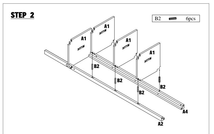
Attach the rest of Shelves A1 to Legs A2 & A4 using Wood Dowels B2 as shown above.
