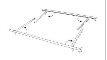
**Step 2** Place rivets of the cross arms and extension bars into appropriate key holes then slide to lock as shown in Figure 1. Secure extension bars with the four bolts provided as shown in Figure 2.
