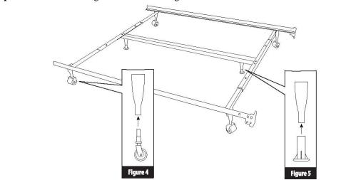
**Step 5** Put the plastic corner pad to the end of the side rails shown in Figure 5
