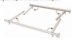
**Step 2** Place rivets of the cross arms into appropriate key holes then slide to lock as shown in Figure 1. The extension bar is not required.
