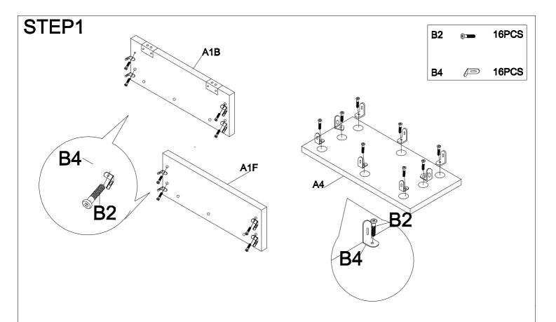
Attach Brackets B4 to Front Panel A1F,Back Panel A1B,Bottom Panel A4 using Bolts B2.(Please do not tighten Bolts B2 unit Step 3.)
