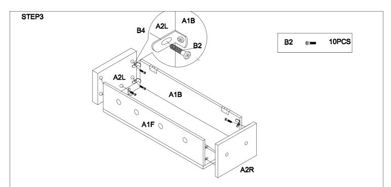
Assemble Side Panels A2L&A2R to Front Panel A1F and Back Panel A1B,Bottom Panel A4 using Bolts B2. Then tighten all bolts at this point.
