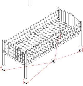
Please Check Bolts regularly during use, if any bolts loosen, please tighten it right away to reduce any risk of damage to user or item.
