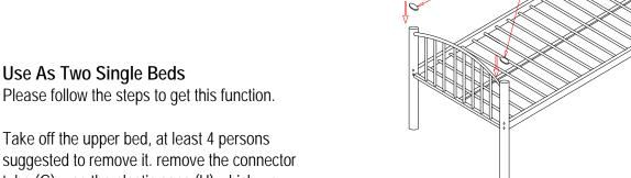
Take off the upper bed, at least 4 persons suggested to remove it. remove the connector tube (G), use the plastic caps (H) which we supplied 8pcs extra in the shipping carton to cap the upper tubes and bottom tubes. see following image. and keep the connector tubes (G) storage away for future use, see right Image shown.
