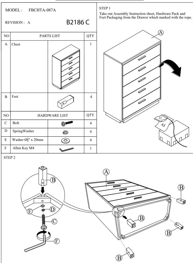
Insert Leg (B) at position as shown and tighten with JCBC Screw (C), Spring Washer (D) & Flat Washer (E) by using Allen key (F)
