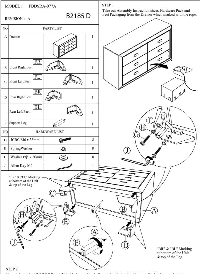
Align & fasten feet (B),(C),(D) and (E) to Unit according to the position left and right follow the label correctly using bolt (G), lock washer (H) and flat washer (I) and fully tighten with Allen Key (J). Align and tighten Support Leg (F) with leveler to bottom panel of unit (A) by turning center feet with leveler clockwise until tight.
