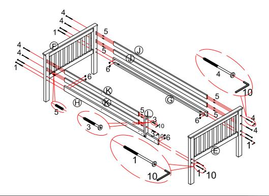
Attached guardrail reinforce bars (M) to back guardrail bar (J), front guardrail bar (K), front upper side rail (H) and back upper side rail (G) with bolts (2).
