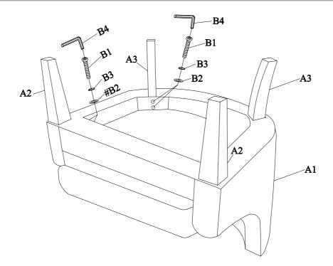
Attach Front Legs A2 and Rear Legs A3 to the bottom of Seat A1 using Bolts B1 with Flat Washers B2 & Spring Washers B3 as shown above, do not tight bolts until all bolts until Step 2.
